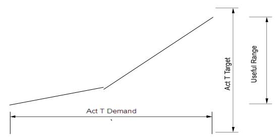
Act T Demand, is derived from Act T Demand raw, the Pedal and input from the idle speed controller shown in Act T Idle mod. The calibration defines 3 different relationships between demand and target in the tables: Act T Target, Act T ALS Target, and Act T ALS Mild Target, these are selected with the ALS modes. Useful Range limited by Act T Target max and Act T Target min.
