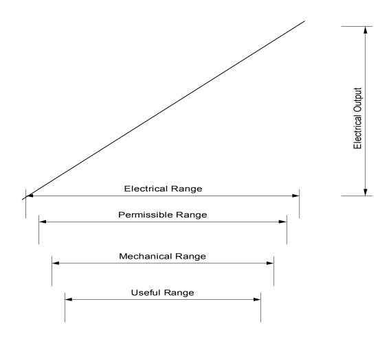
Permissible range defined by **Pedal Max** and **Pedal min**, measured with Pedal raw, a combination of both duplicated pedal position sensors. If out of range then flag *Error Pedal* = *On*, and **Pedal Default** active in place of normal control. Useful Range defined by **Act T Pedal max** and **Act T Pedal min**, to produce *Act T Demand raw*.
