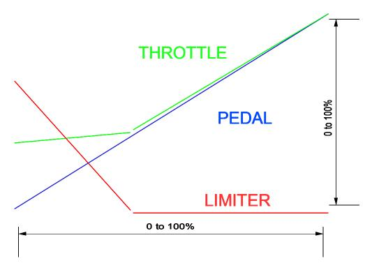
With Anti-Lag turbo boost enhancement, the throttle is open even with no accelerator pedal depression. There is an effective gap between throttle and pedal, this must be accommodated with the limiters. The limiters will consist of a combination of fuel cutter, spark cutter, and ignition retard, often some additional fuel is required.
