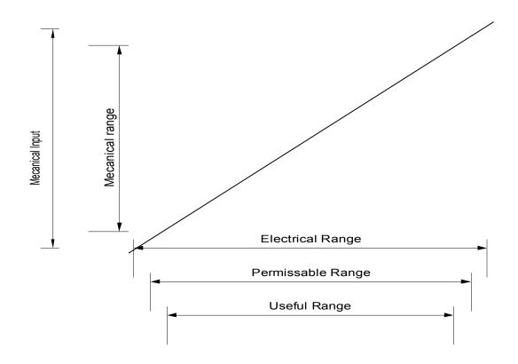
Electrical Range is shown in *Act T Position*, and compared with *Act T Target* to derive *Act T error*, for the controller.
